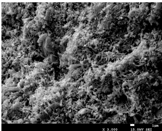
(c) SEM diagram after 72h curing of the refined mixture two of the nano-composite cement ( \times 3000 , \times 5000 )
