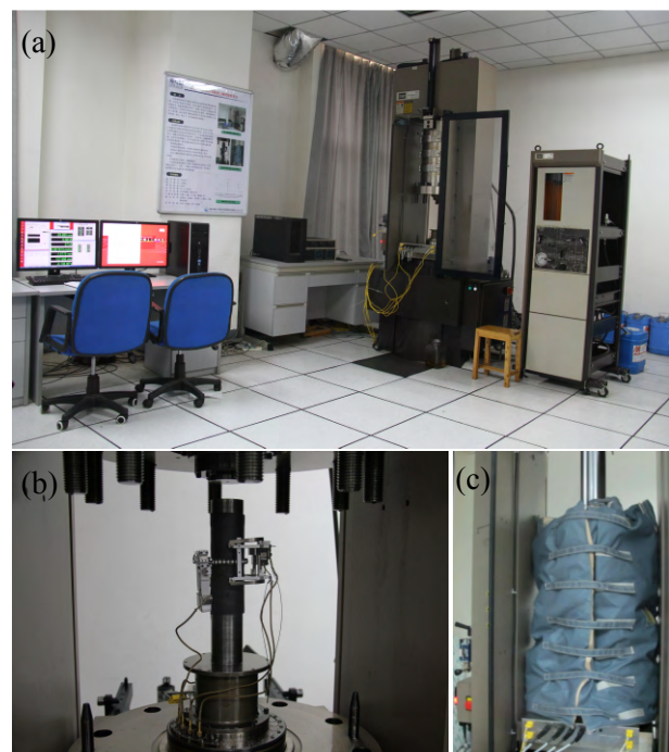
Figure 1 MTS 815.03 triaxial test equipment. (a) Total view; (b) The equipment used to measure lateral and axial deformation; (c) The arrangement for heating and keeping at constant temperature of the samples.
