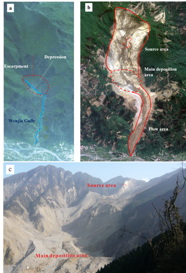
Figure 10. Sketch map of flow capacity of channel affecting on the travel distance of the Wenjia Gully channelized rock avalanche: (a) before the earthquake; (b) after the earthquake; (c) photo taken on deposition platform after the earthquake. The red arrow shows the sliding direction of source mass. The red dotted line in (a) indicates the original depression on the travel path of the rock avalanche, where debris deposition of about 30 million \text{m}^3 was stored after the earthquake (shown in b); more detailed information is shown in (c).
