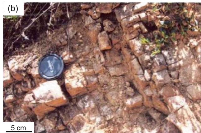
Fig. 4 a Stereonet graph of rock mass discontinuities in the source area ( J_1 tension joints; J_2 compressive joints). b Fragmentized basaltic rock mass in the source area
