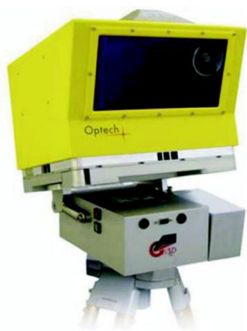
Fig. 4 ILRIS-3D scanner on tripod for different angles
