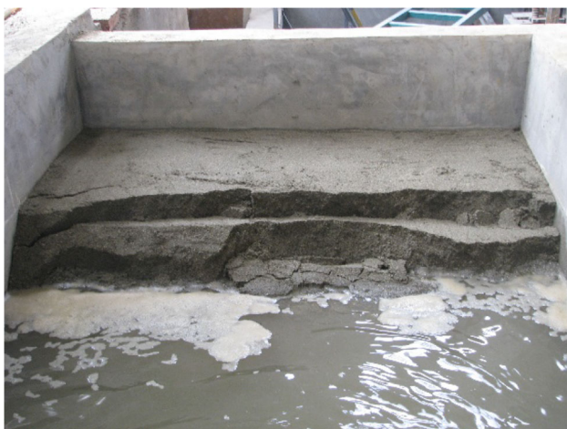
Fig. 3 Collapsed model in physical simulation flume
