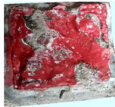
Fig. 12. Morphology of Structure Surface after Shear Test
