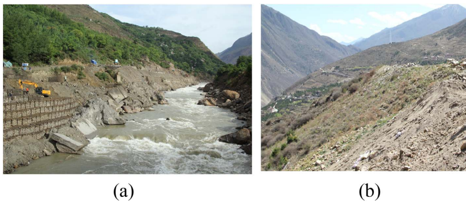
Fig. 16. Photos taken during field surveys. (a) The Dajinchan River at the foot of the Jiaju landslide (May 2015); (b) Waste soil dumped at the rear part of the Jiaju landslide (April 2017).
